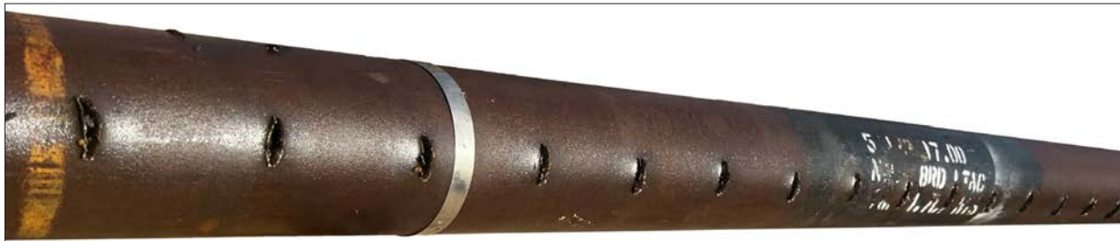
3-1/8" 5.14SPF, 15' GUN, PHASING 0°-180°, 5° SLOW ROTATION, CENTRALIZED IN 5-1/2" 17# L-80 CASING, AVERAGE SLOT SIZES: 1.37" LENGTH X 0.21" WIDTH
