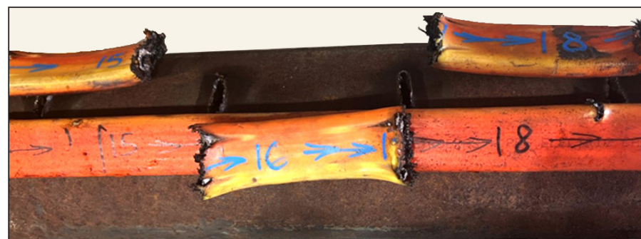
FLAT PACK DIMENSIONS (PRE-TEST): 1.417" x 0.55" TESTED WITH 3-1/8" 5.14SPF IN 5-1/2" 17# L-80 CASING
