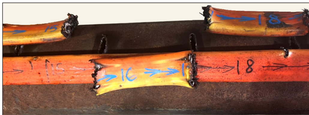
FLAT PACK DIMENSIONS (PRE-TEST): 1.417" x 0.55" 3-1/8" 5.14SPF IN 5-1/2" 17# L-80 CASING (SEVERED FLAT PACK IS ~4.67" IN LENGTH)
