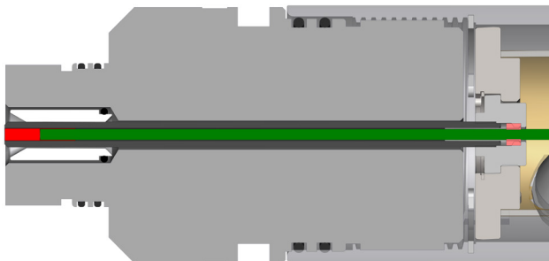
Transfer kit components installed in top sub with detonator and detonating cord.
