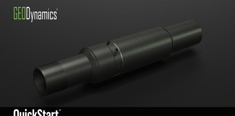
The GEODynamics QuickStart™ Inject + Frac Valve provides the operator with an initial point to break down the formation and establishes a pump-in port for use in long horizontal completions. The device is comprised of an opening piston that is controlled by a special rupture disc.
